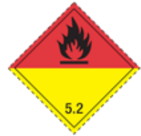
(No. 5.2) Class 5.2 Organic peroxides Symbol (flame): black or white Background: upper half red; lower half yellow Figure '5.2' in bottom corner
